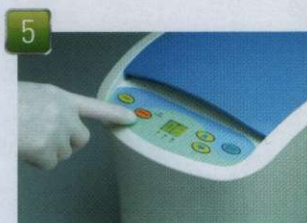
Press down the key "ST/STOP" to start running.
