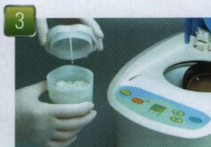
Close tightly the cap of mixing bowl.
