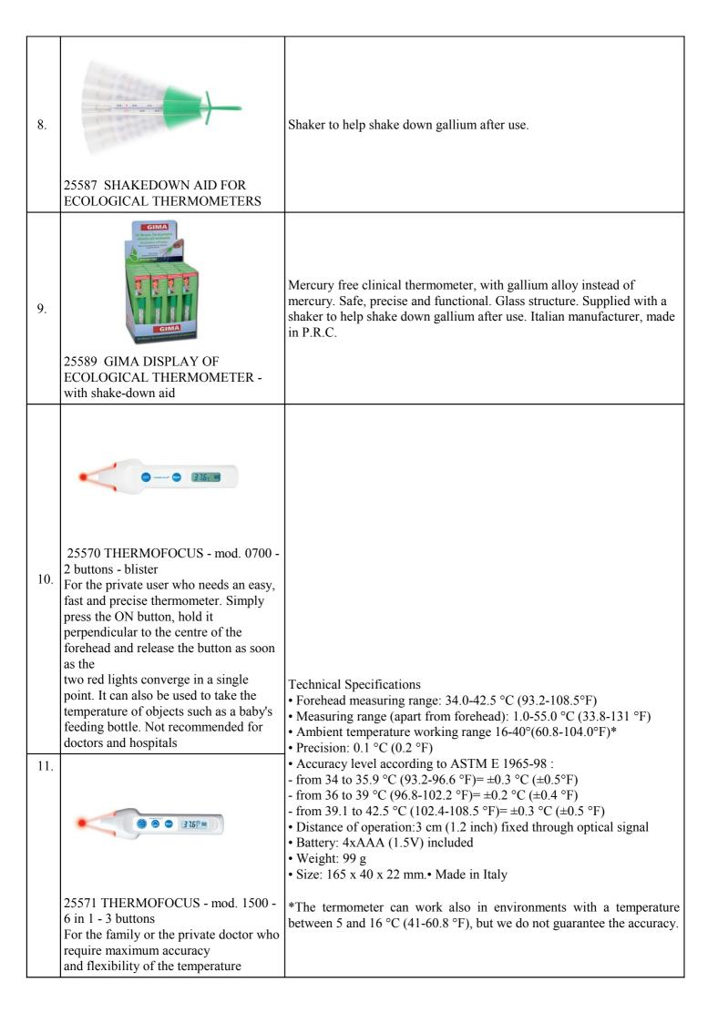
taking. Same as 25570 with an additional button ("home") to read the ambient temperature and that of other parts of the body (such as navel or armpit), as well as the temperature of objects and liquids within a range from 1 to 55 °C (33.8 to 131 °F). Provided with the exclusive Manual Quick Calibration System (MQCS) technology through which the thermometer is always perfectly stabilized to the ambient temperature.
